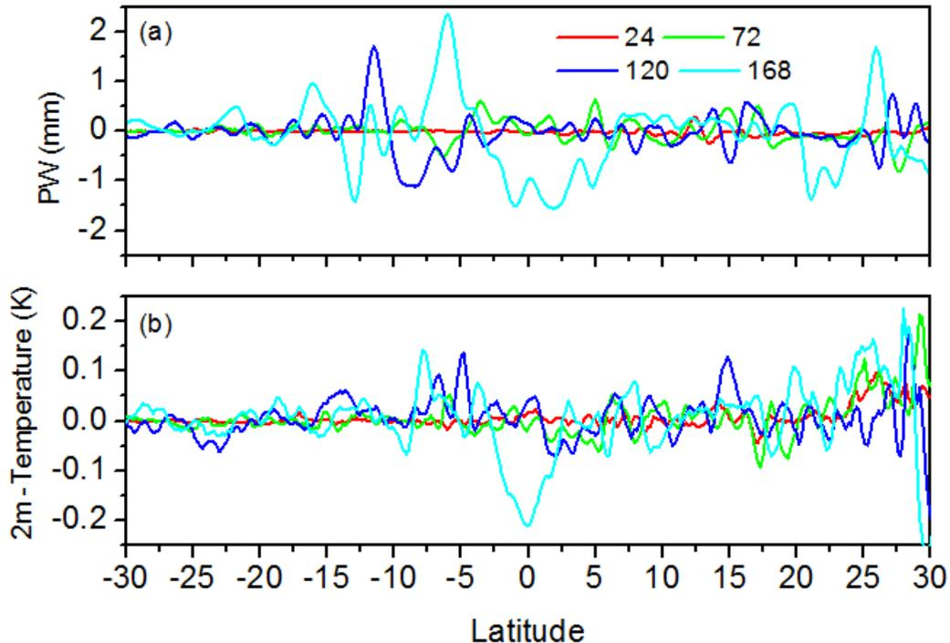
Figure 12: Composite plot of (a) difference of precipitable water (mm) and (b) 2m Temperature (K) over tropical latitude, averaged over Indian longitudes (70-90 E). The colour legend indicates the forecast hours.
