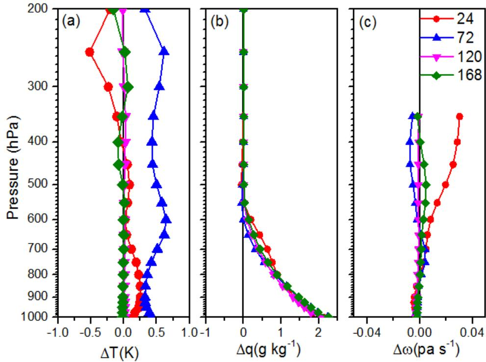
Figure 7: Vertical profiles of difference in (a) temperature, (b) specific humidity and (c) vertical velocity over region (a) of Indian land mass between cold bias correct experiment and GFS.
